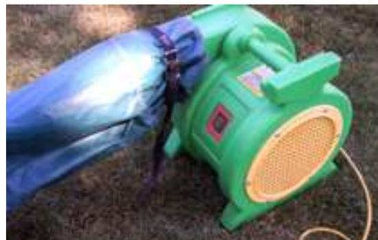
6. Twist the vent (the other tube) several times, fold it over and secure snugly with the attached strap.
